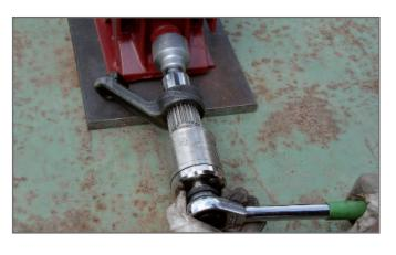
Example: Manual nut-runner with stepdown gearing for easy unscrewing af the loaded hexagonal nut
