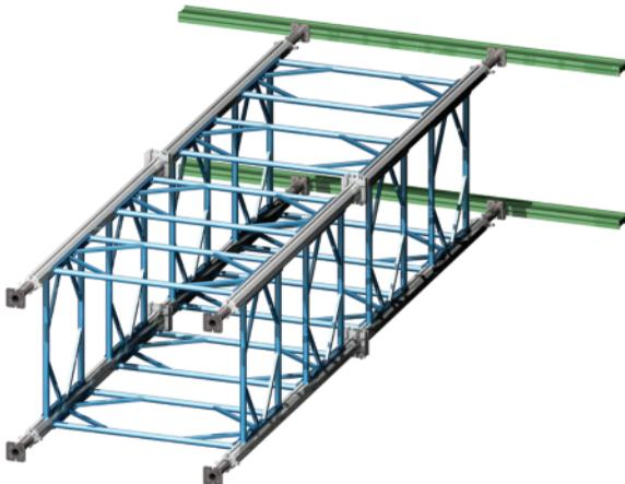
The fixing of the H-frames to the joint of external tube is made quick and uncomplicated with the help of 3 captive bolts per frame side.
