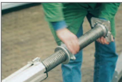
In that way **the adjustment range** of 1.20 m **will double** to 2.40 m.
