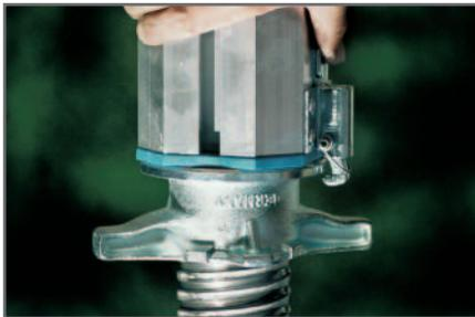
The **spring-loaded safety hook** at the external tube secures the spindle against discharging. For a quick adjustment in unloaded condition this hook can be released. The spindle with the swivelling nut can be removed from the external tube and the swivelling nut can be easily turned.
