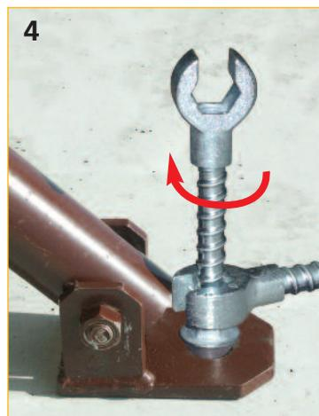
4. Final tightening of the screw by simply turning it with second scrwe-in set. Because of the form of a screw spanner of the scrwe-in set also a conical flange nut can be tightened.
