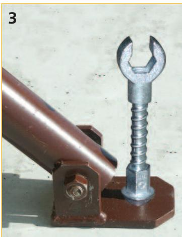
3. Tighten hexagonal nut by hand, in this way the nut will center the clamping part without tolerances.
